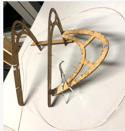
From this point on, we continued to work on part one and two separately. For the upper body, we created the first wearable. This we first prototyped with paper and cardboard. The resulting shape is then laser cut from wood.
